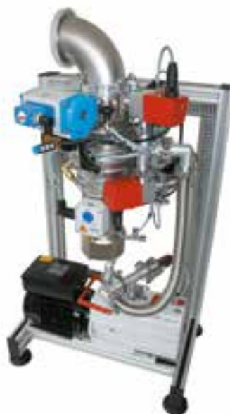
Diffusion pump set mounted on customized rack
